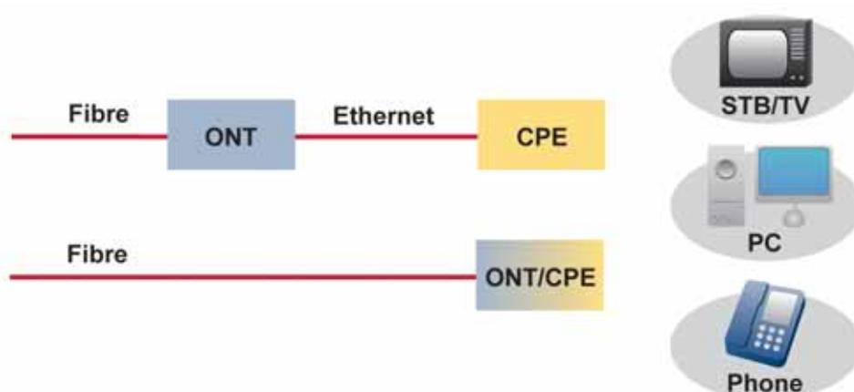
Figure 16: Possible configurations of the ONT and CPE.
