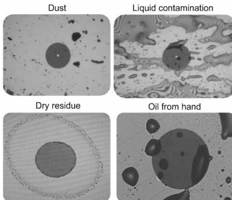
Figure 103: Appearance of various contaminants on a connector end-face.
