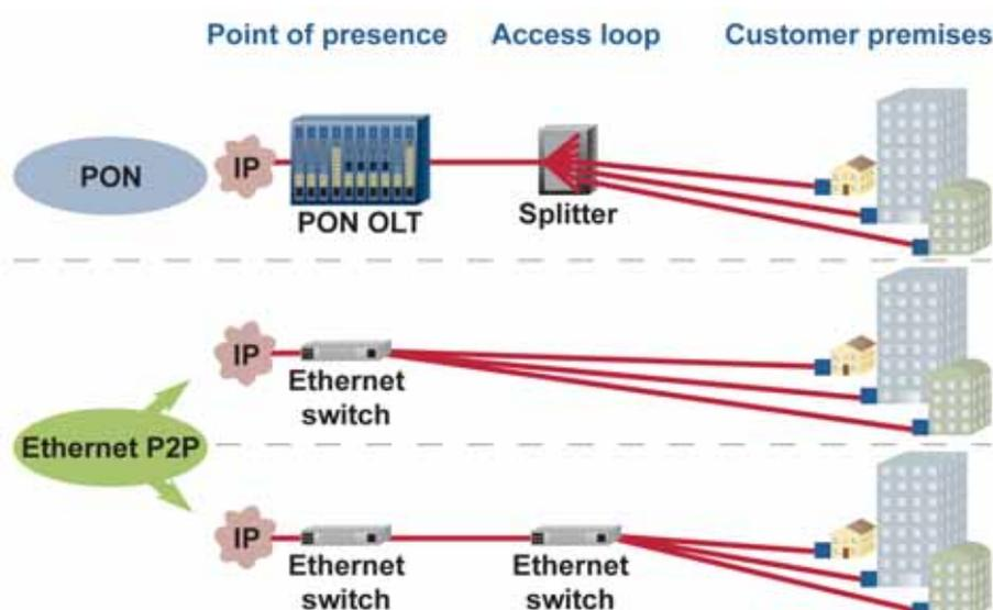
Figure 5: Different FTTH network architectures.
