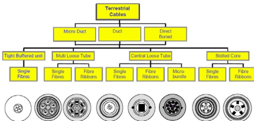
Figure 48: Duct cable selection.
