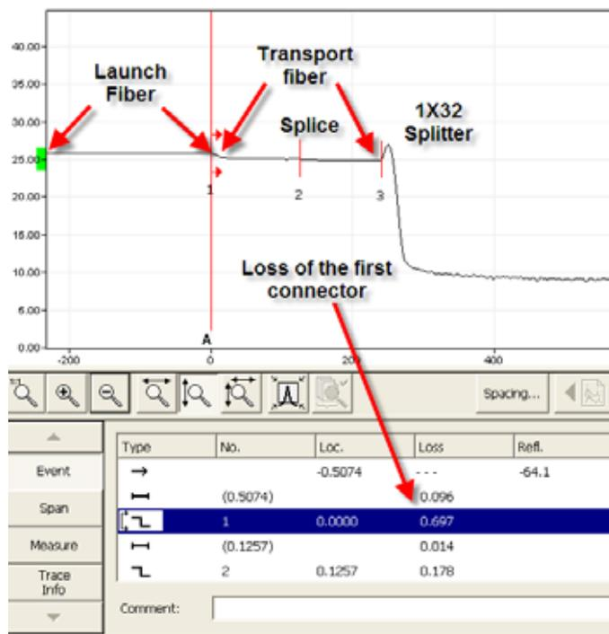
Figure 110: Using a launch fibre makes it possible to characterize the first connector on any segment of your network. A pulse width of 300-500m will be sufficient for this test.
