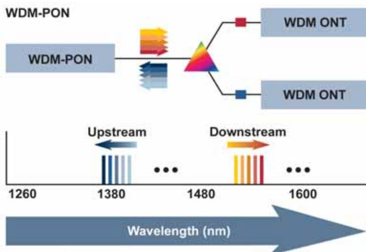
Figure 20: Wavelength plan for WDM-PON
