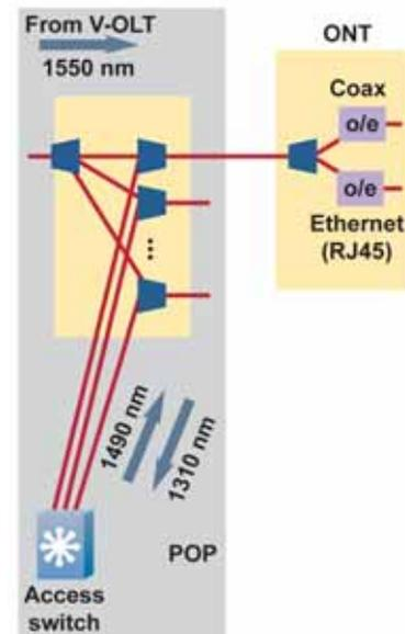
Figure 15: Insertion of RF video signal into point-to-point fibres.
