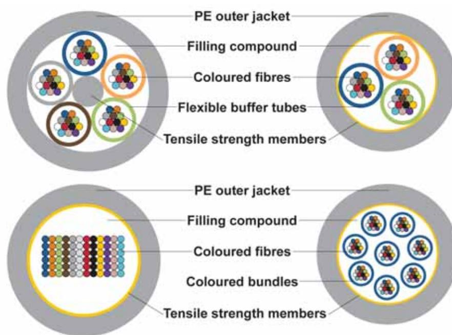
Figure 63: Microduct optical fibre cables (not to scale).
