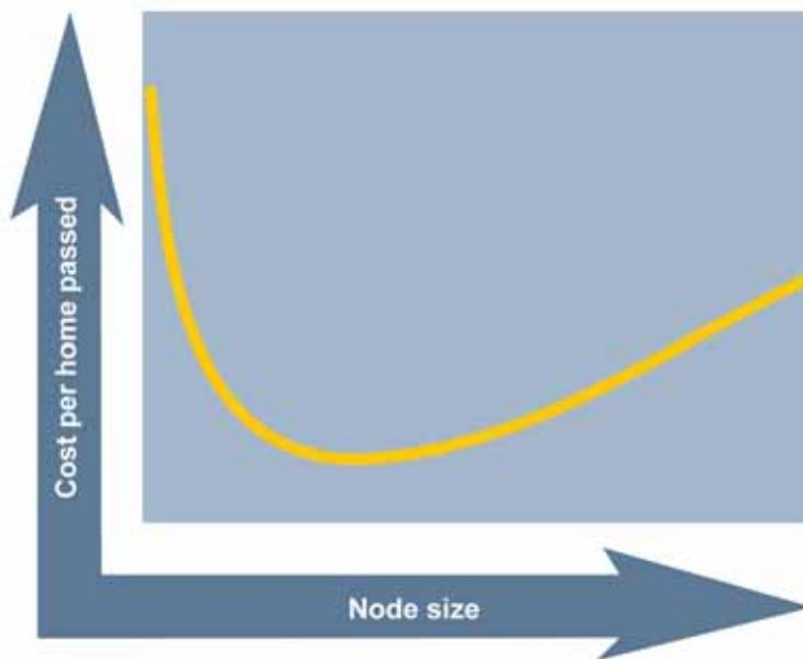
Figure 10: Optimisation of node side in a PON with single-level splitting
