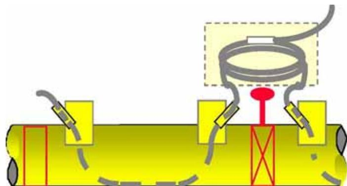
Figure 78: Gas pipeline section, including I/O ports and the bypassing of a valve defining one point-of-presence for the fibre optic cable.
