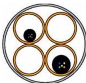
Figure 46: 110mm main duct with four rigid subducts.
