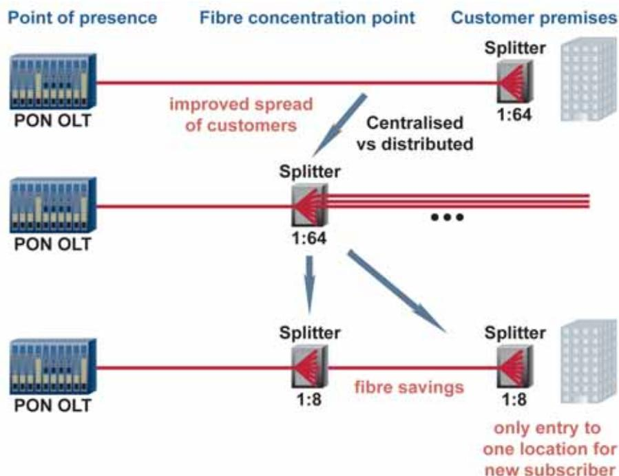
Figure 11: Centralized and distributed splitting in a PON
