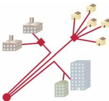
Figure 3: Active Ethernet network.
