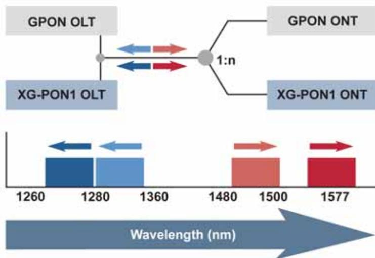
Figure 7: FSAN approach to XG-PON
