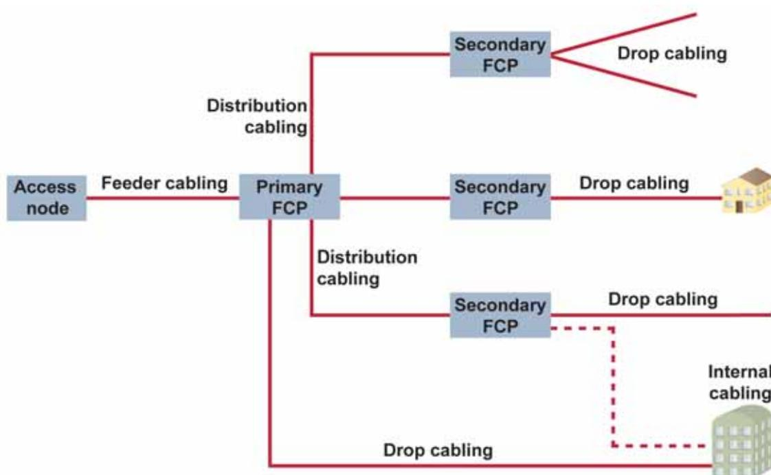
Figure 23: Main elements in a FTTH network infrastructure.
