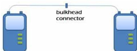
Figure 107: Test sets should be referenced prior to measurement.
