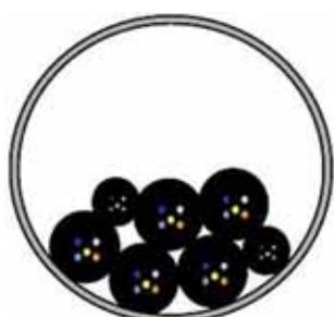
Figure 45: 110mm main duct.
