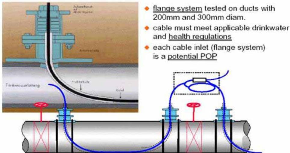
Figure 79: Cross-section showing fibre installed in a drinking water system.
