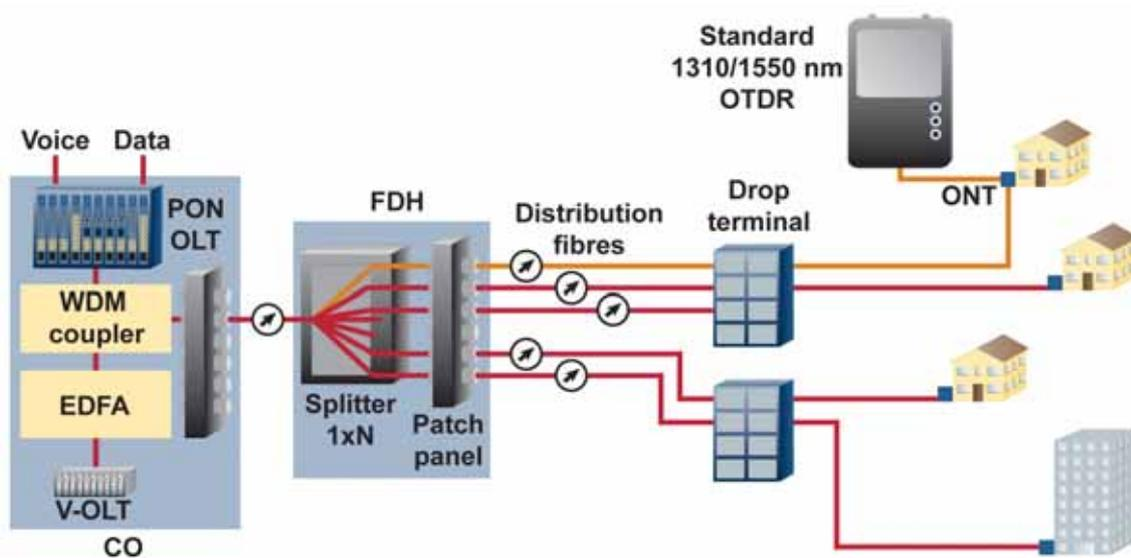
Figure 109: Measurement with an OTDR.
