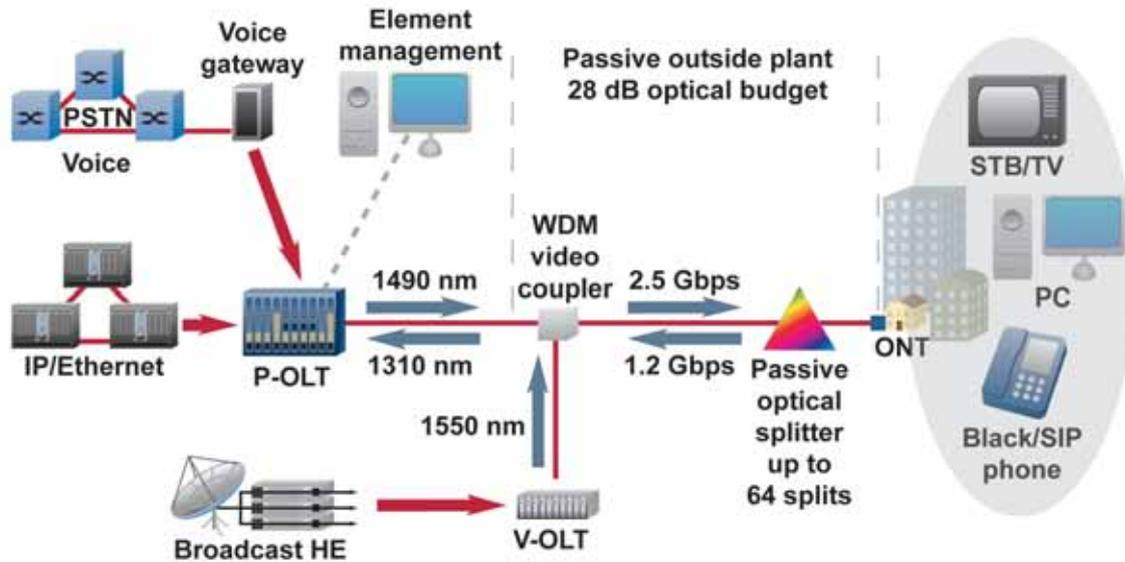
Figure 6: Schematic diagram of a GPON network.
