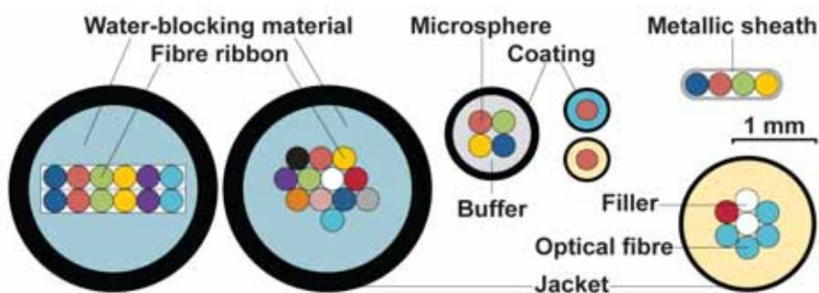
Figure 65: Examples of Fibre units.
