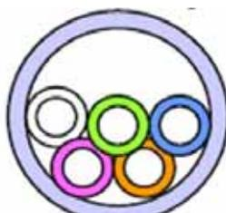
Figure 54: Post-installed microduct.
