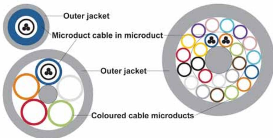
Figure 64: Protected cable microduct with tight integral outer duct (not to scale).
