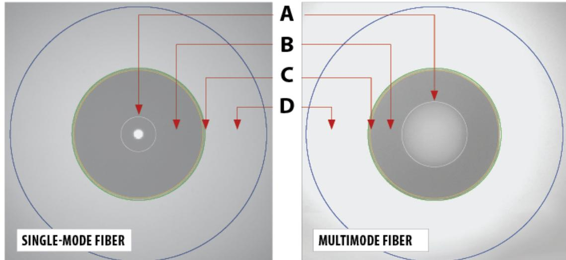
Figure 102: Connector end face inspection zones
