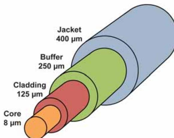
Figure 86: Optical fibre construction.
