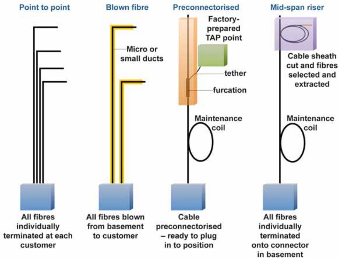
Figure 34: Different schemes for MDU cabling.
