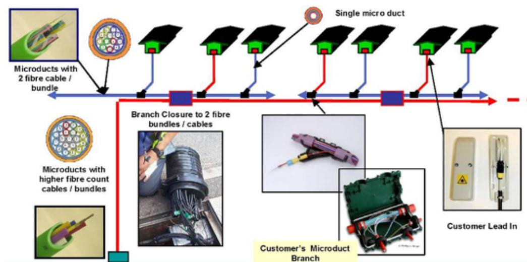
Figure 52: Product map for blown microducts and microcable.
