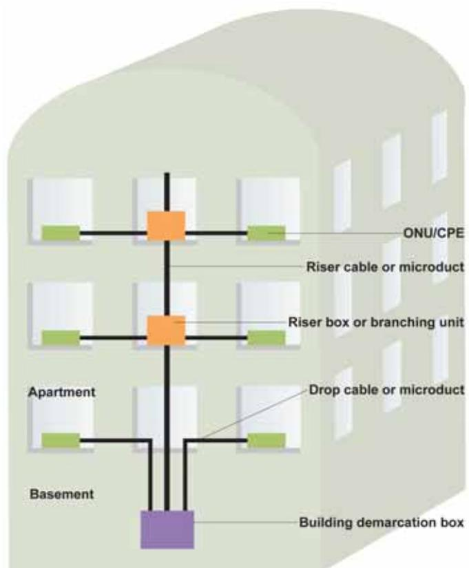
Figure 35: Options for internal cabling of a building.
