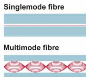
Figure 87: Light paths inside fibre.
