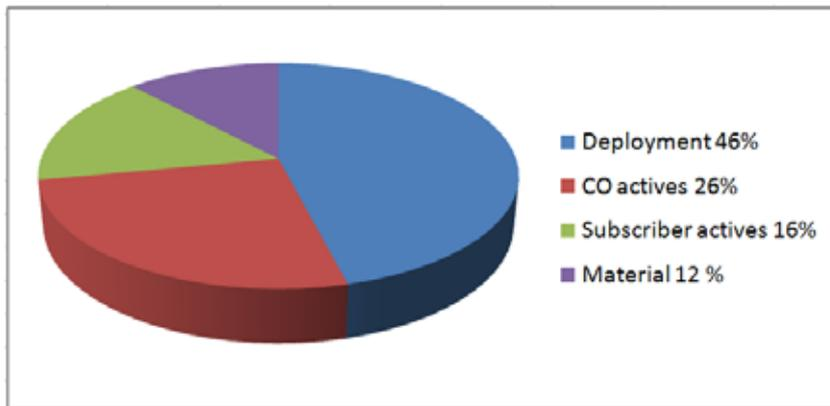
Figure 22: Typical initial CAPEX distribution for Greenfield FTTH deployments.
