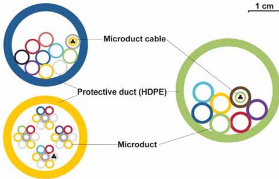
Figure 62: Protected microducts with loose package.
