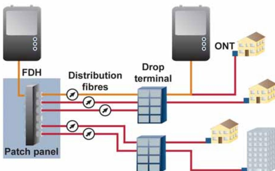
Figure 108: Measuring distribution fibre IL and ORL using a pair of OLTS.
