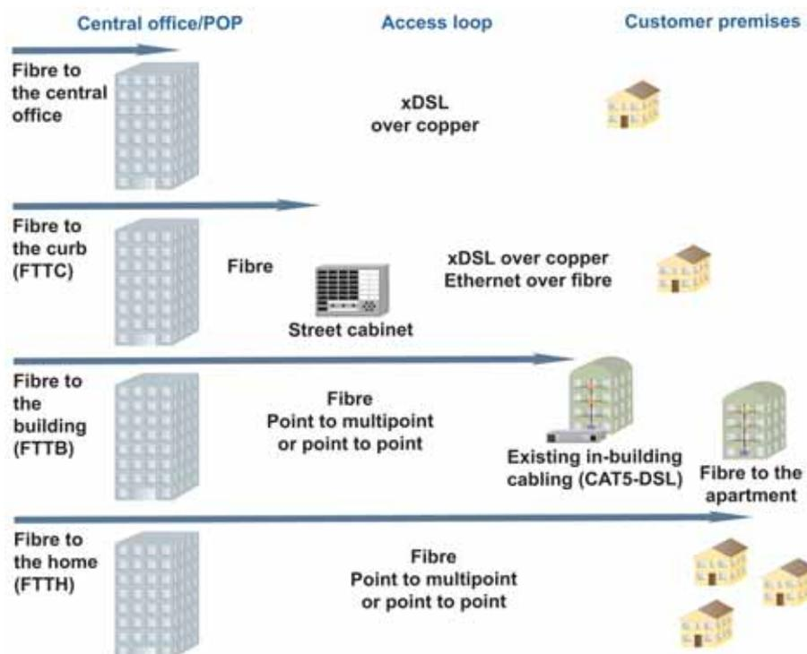
Figure 4: Different types of FTTx networks.
