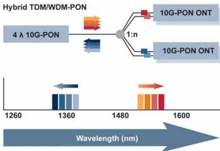
Figure 21: Wavelength plan for hybrid TDM-WDM-PON
