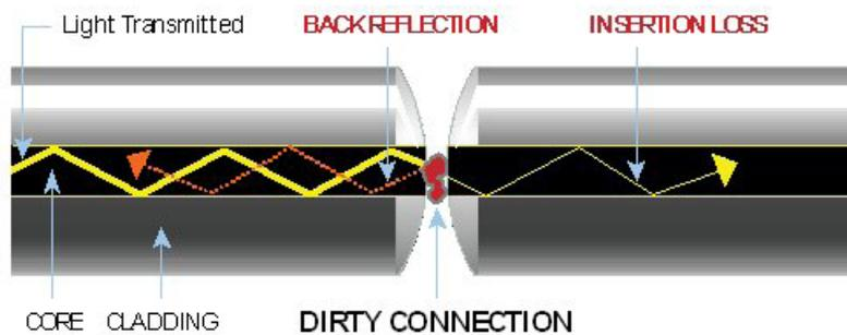
Figure 101: Increased insertion loss and back reflection due to dirty fibre connection.
