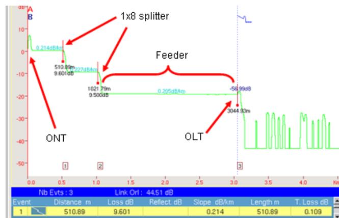
Figure 111: PON optimised OTDR test from the ONT to the OLT.
