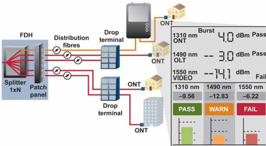
Figure 113: Pass-through testing of all wavelengths.
