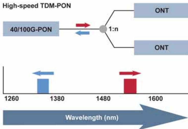
Figure 19: Wavelength plan for TDM-PON
